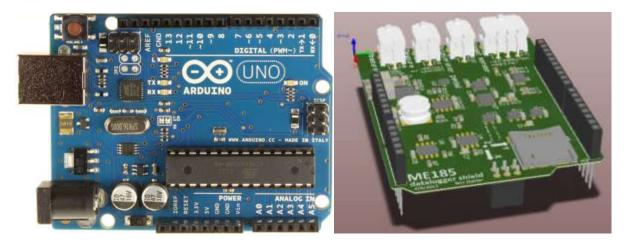
The datalogger is based on an Arduino Uno (<a href="http://www.arduino.cc/">http://www.arduino.cc/</a>) and a custom datalogger shield. The datalogger shield contains a SD socket, a 3 axis accelerometer, a 3 axis gyroscope, a switching power supply and signal processing circuitry for battery voltage, battery current and speed sensor measurement.
