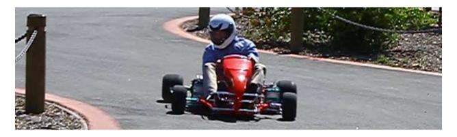
The Go-Kart was built by an ME185 team in 2012. The kart is equipped with 40Ah lithium batteries and a 6Hp (continuous) brushless motor. The chassis is designed for a shifter kart.
